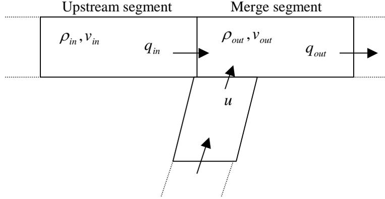
**FIGURE 1** Ramp system (upstream segment, merge segment, and ramp link).
