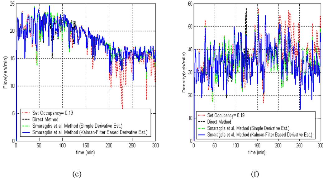
**FIGURE 3** Comparison of the proposed methods with method suggested by Smaragdis et al. (2004) for sudden drop of the critical density (Figures 3a and 3b), gradual drop of the critical density (Figures 3c and 3d), and flow and density vs. time plots for gradual drop of the critical density (Figures 3e and 3f).
