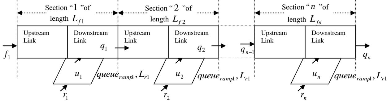
Fig.1. “n” freeway sections with one on-ramp.
